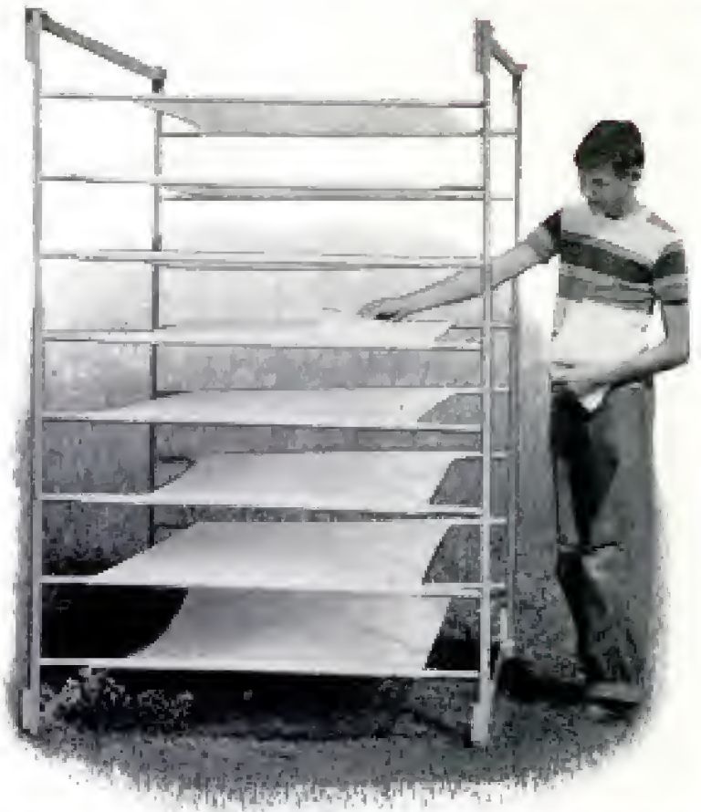
Drier can be set up indoors or out and can be made larger or smaller to suit requirements. Fabric "shelves" are 36 in. wide
